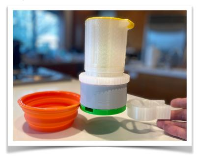
3D PRINTED DOG FEEDER WITH CUSTOM WHEELCHAIR MOUNT (ON RIGHT) AND EMBEDED ESP-32 CONTROLLER (LISTENING OVER BLE AND MQTT). (PRODUCT CALLED PETTUTOR FROM <u>SMART ANIMAL</u> <u>TRAINING</u>).
